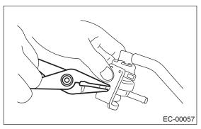
10) Disconnect the pressure control valve hose from pressure control solenoid valve.
