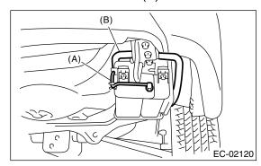
7) Remove the canister from vehicle.
