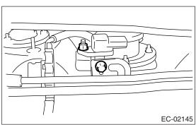
6) Disconnect the pressure hose from fuel tank pressure sensor.
