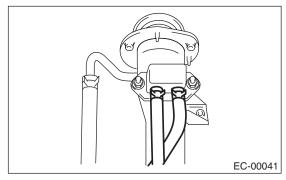
3) Remove the shut valve from fuel filler pipe.
