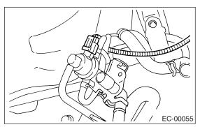
8) Disconnect the two evaporation hoses from pressure control solenoid valve.
