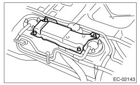
3) Remove the clips, and disconnect the hoses from vent valve.
